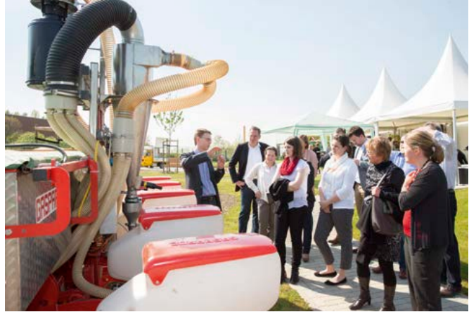
SweepAir is a prototype technology based on a cyclone system that separates the dust from the outlet air of vacuum-pneumatic planters.
