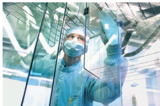
Bayer employee Michael Delbeck prepares polycarbonate sheets for the application of a scratch-resistant coating.
