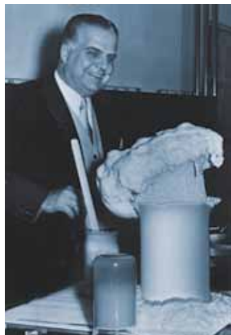
Bayer researcher Dr. Otto Bayer experimenting with the foaming process for polyurethane
