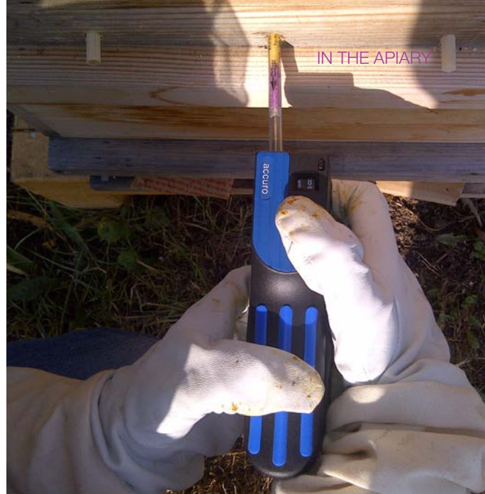
To find out how formic acid distributes in the beehive, the researchers drilled holes into the chest and measured the acid concentration at different locations inside.
